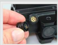
In order to use the mini-dongle, unscrew switch button B1 and place the mini-dongle on the screw thread.
