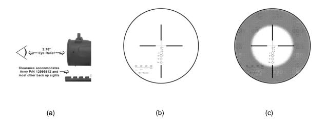
Figure 2-2 (a) Eye shown at proper 2.75 inch eye relief distance from rearmost glass surface. (b) Image through sight is sharp and circular when eye is placed at or near the proper eye relief distance. (c) Image through sight when eye is too close to or too far from optimal viewing distance.
