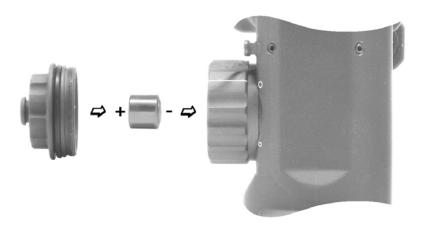
Figure 2-7 Battery replacement
