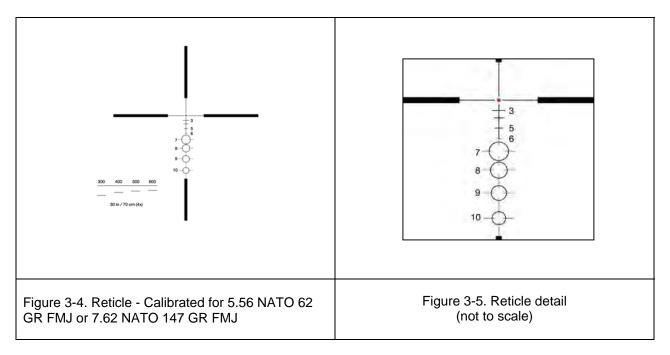
The reticle of the Optical Sight provides the shooter with easily located aiming marks to designate the target at both short and long ranges.
