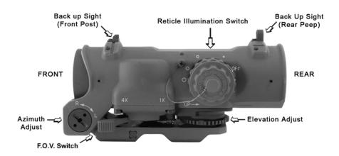
Figure 1-2 Left Side View and Selected Controls
