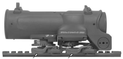
To fully disengage the ARMS levers, rotate them to a position 90° with respect to the sight body. Place sight onto rail as shown. Close levers to lock sight onto rail.
